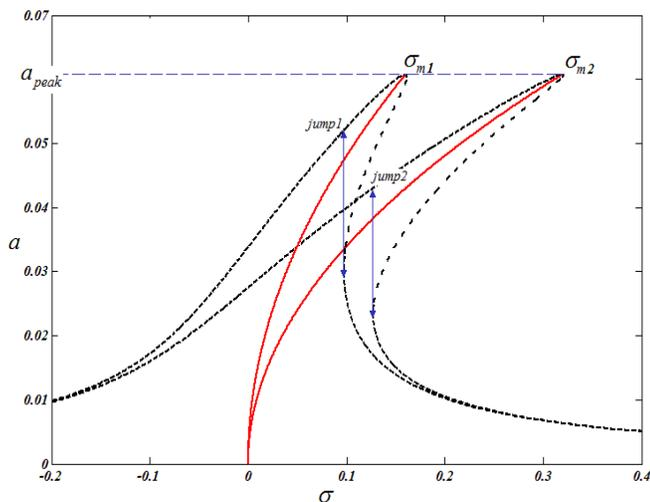
Figure 2: Frequency response of system for two typical cases
