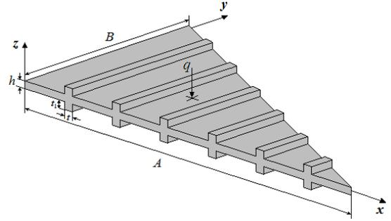
Figure 1: Schematic model of a triangular-shape plate with six stiffeners and excitation load  $q$
